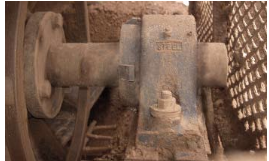
The plant was sold on Blue Brute bearings, made by QM Bearings. The bearings lasted four times as long as the previous bearings from a competitor despite the gravel, sand and water contamination.
