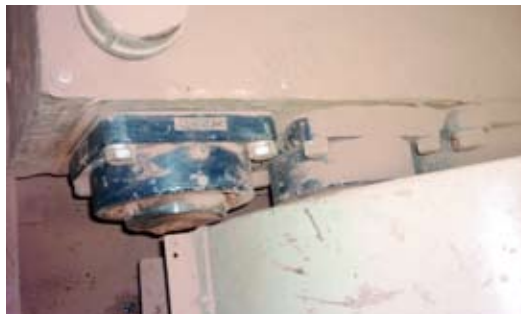
Another type of Blue Brute bearing, flange mounted, is used on the brick manufacturer even feeder.
