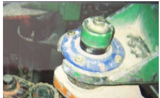
AM Blue Brute bearings stand up to the high shock loads on the Denis Comact log turner.
