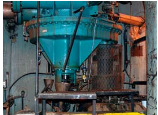
The QF10260 Quick-Flex spacer couplings have run for 10 years on three applications, including this Kamyrdigester outlet device, without the need to replace an original insert.
